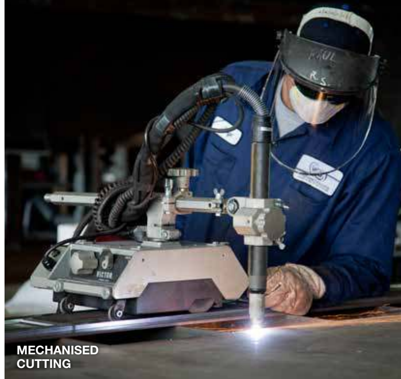
DRAG SHIELD CUTTING
